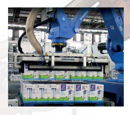
The UniGripper LayerGripper is offered as a complete system including selected side channel blowers for vacuum generation and smart solutions for the installation of the vacuum hose.
